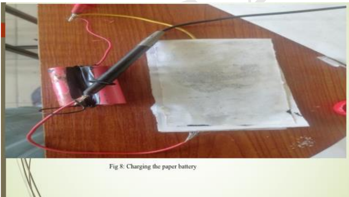
Fig 5. Charging the battery
